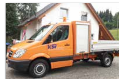
Tool box fitted with roller shutters
