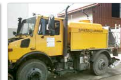
Retrofitted road-rail vehicle
